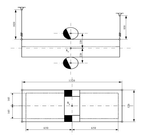
Fig. 1. The basic dimensions of the experimental screen
